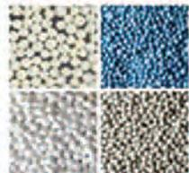
To achieve alternative dew point the Sullair dryer uses a mixture of absorption media "Molecular Sieve" or "Silica gel application."
